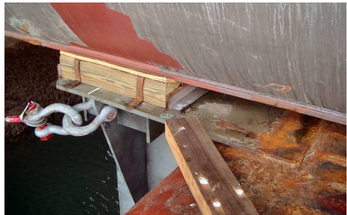
Figure 11. Port aft cribbing block compressed after lifting rig.
