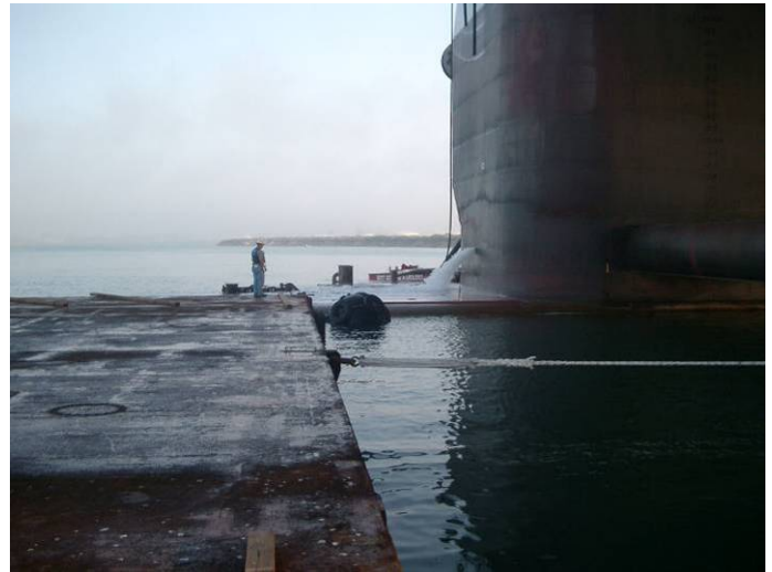
Figure 10. Barge pulled in between rig pontoons.
