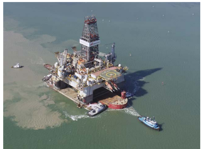
Figure 1. Tow-out of the GSF Development Driller I with a lift from Boabarge 16 .
